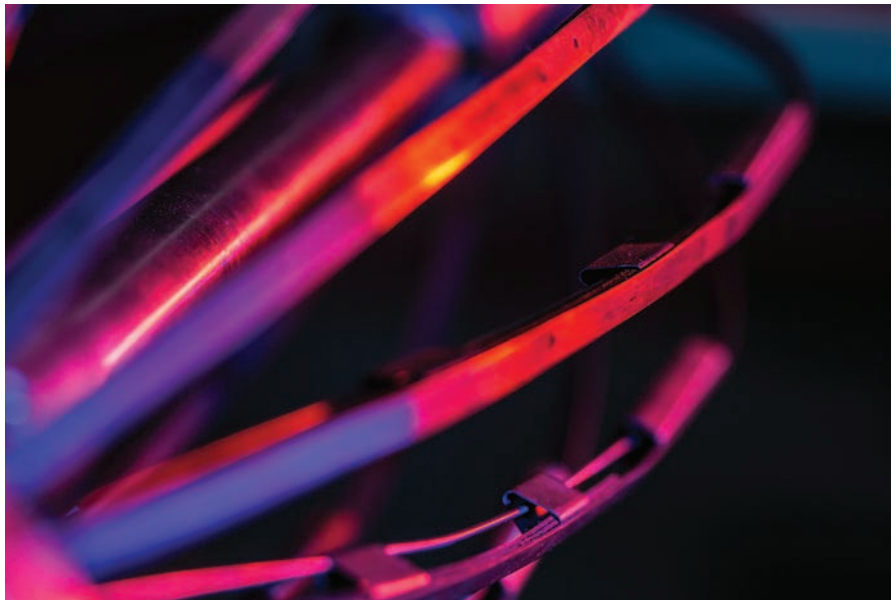
READ Cased Hole notes that increased activity on the UK Continental Shelf is creating scope for expanding the business. Pictured is an abstract image of a spinner array which is run as part of a production logging tool string and specifically identifies individual fluid velocities
