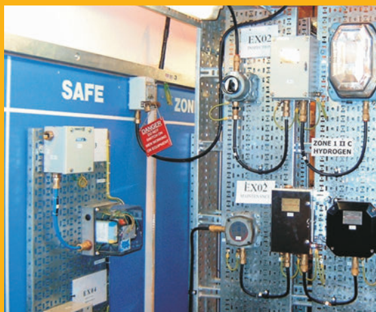
Part of a CompEx Practical Assessment Rig – the CompEx Scheme is founded upon practical training and assessment to validate core competency
