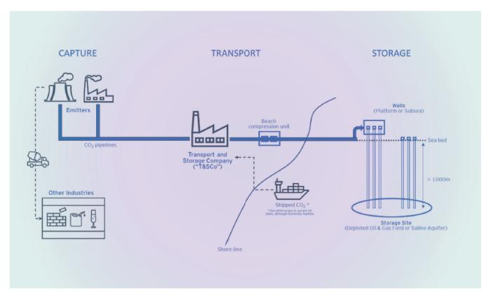
CCS is an integrated chain of technologies and systems, consisting of Capture, Transportation, and Geological Storage of CO<sub>2</sub>.
