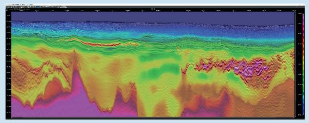
Inline: Phases 1 & 2 – full stack with velocity overlay
