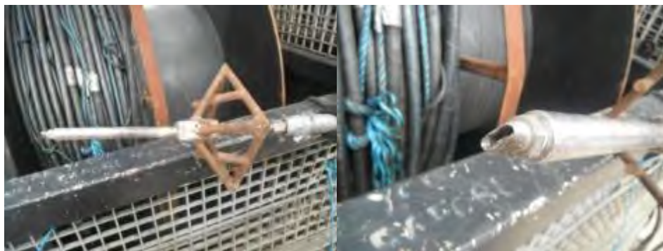
Figure 7-5 ROV crew jetting lance and bespoke nozzle
