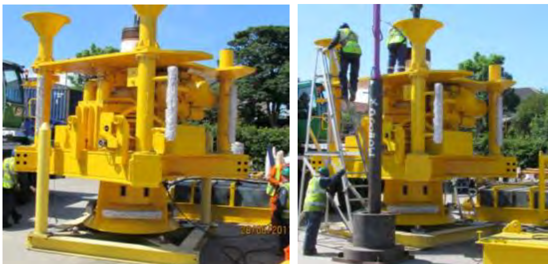
Figure 6-9 EERD Cap shipping skid with and without guide post clash
