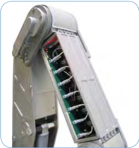
Slave arm electronics are located in the forearm, increasing system reliability and minimizing electrical connections.
