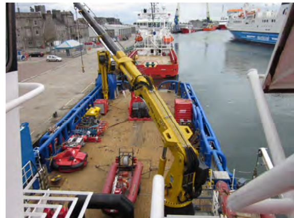
OSR Equipment Secured for Sea
