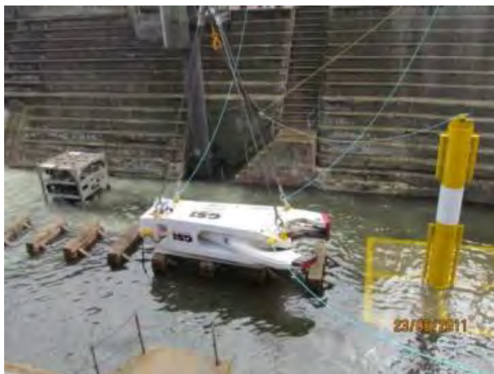
Figure 6-5 GSI Subsea Shears – Cutting Sequence
