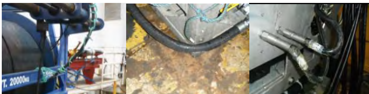
Figure 7-13 Damage to SHPU sustained during recovery
