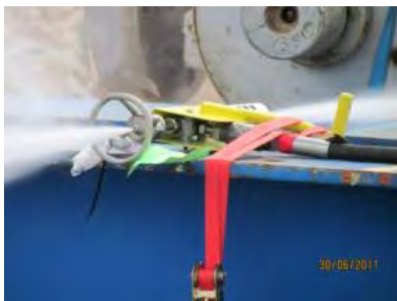
Figure 6-11 ROV Jetting and diffuser unit in action
