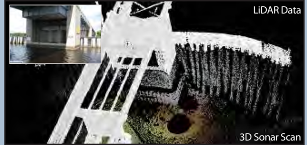
Full View Imagery - easily add underwater details to above-water laser scan data for full, detailed 3D viewing of structures, objects and sites.
