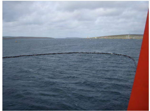
Ro-Boom in "U" Formation
