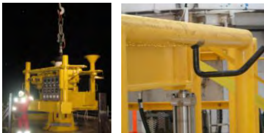
Figure 7-8 Guide Wireless EERD Cap and Bull horns on Landing Base
