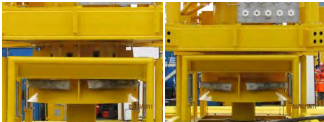
Figure 6-8 EERD Cap caught up on an internal shoulder & fully landed
