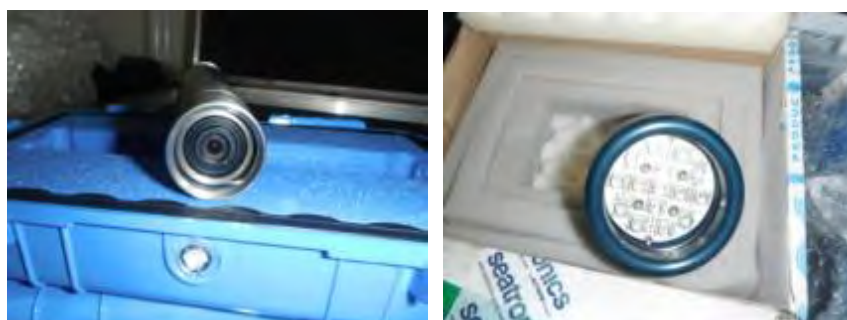
Figure 7-6 L3C-550C Camera and LED - 1600 Light
