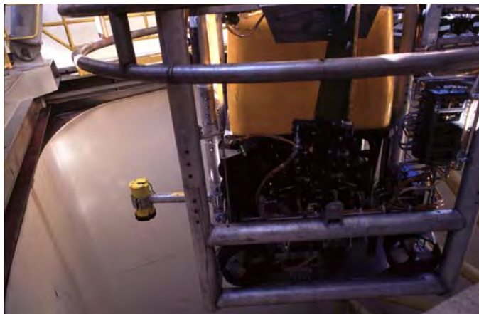
ADCP attached to ROV cage
