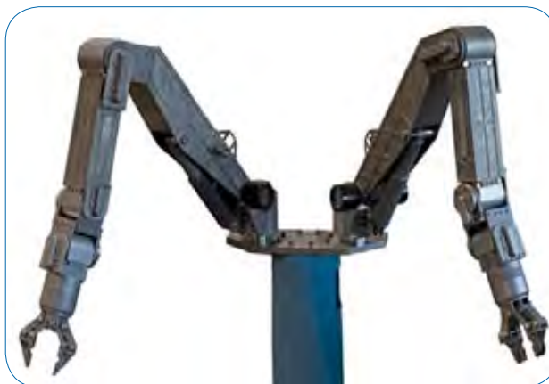
Dual TITAN manipulator configuration.
