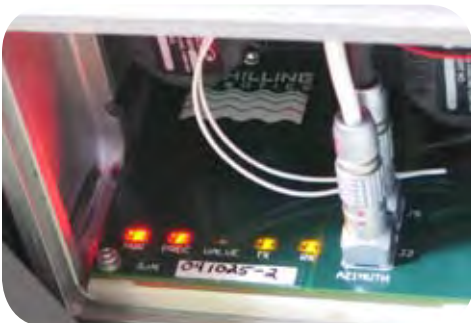
The in-arm slave electronics module features diagnostic lights that indicate processor health.
