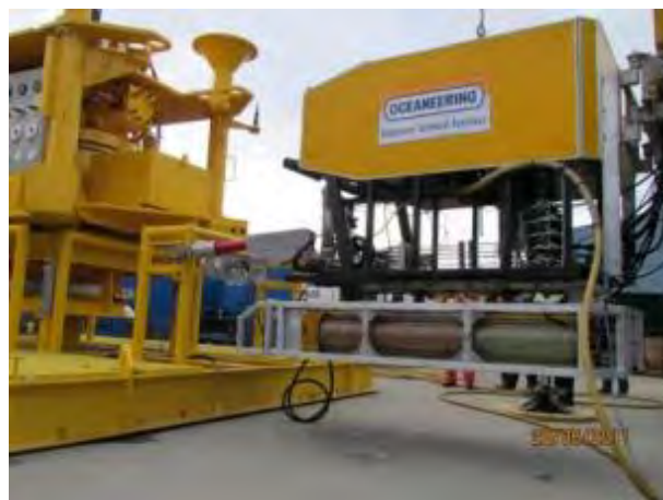
Figure 6-7 Interfacing the pre-loading Structure to the EERD Cap Landing Base
