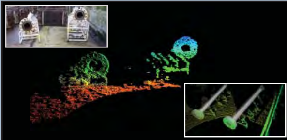
Modeling, Rendering, and Object Identification - improve efficiency and save time by using common laser scanning measurement techniques underwater.
