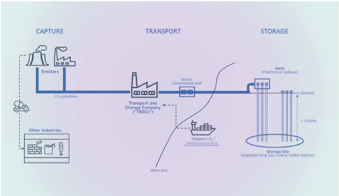
CCS is an integrated chain of technologies and systems, consisting of Capture, Transportation, and Geological Storage of CO<sub>2</sub>.
