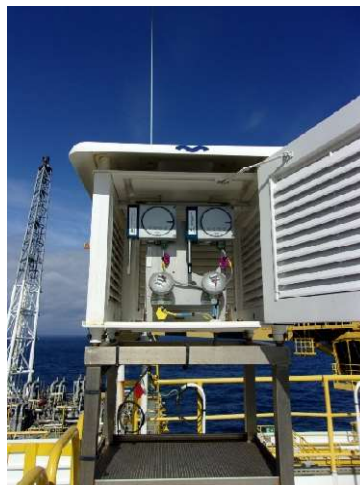
Figure 81: Pressure sensors within a Stevenson Screen
