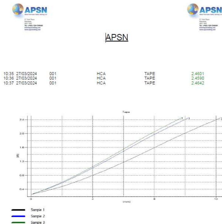
Figure 74: Tensile test of Helideck Perimeter netting Pass and Fail test results.
