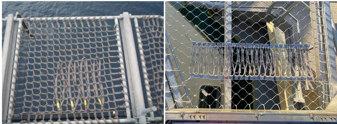
Figure 72 & 73: Perimeter Netting showing Test Strips (kits) used for testing.
