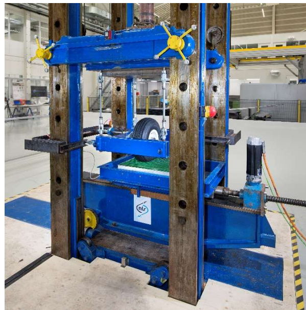
Figure 61: Testing the friction coefficient on a sample of a helideck surface.
