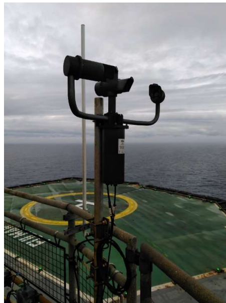
Figure 83: Present Weather and Visibility Sensor
